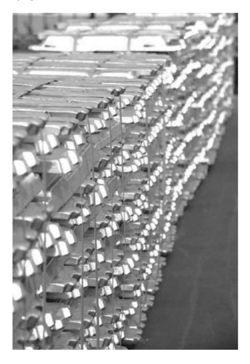
Sales of aluminum alloy ingots accounted for approximately 25.5%, 27.9%, 16.9% and 12.8% of our revenue generated from aluminum products for 2011, 2012 and 2013 and the six months ended June 30, 2014, respectively. Molten aluminum alloy is processed into aluminum alloy ingots through molding, casting and cooling. Our aluminum alloy ingots are produced by using self-manufactured molten aluminum alloy.
